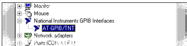
Figure 2-15. GPIB Interface That Is Working Properly
